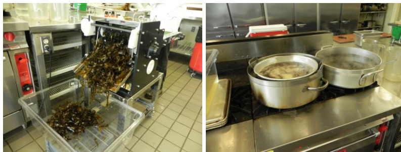
Figure 12. Kelp processing machine cutting the blades and the blanching process.
